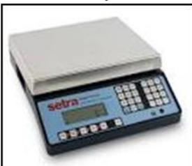
A patented variable capacitance weighing technology lets the scale display weight changes as minute as 1 part in 125,000. The internal resolution, which is four to ten times greater than the display readability, allows operators to work with smaller sample sizes thereby saving time and reducing hand counting errors.
