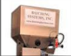
The BSI standard storage hopper has 4 cubic feet capacity providing a backlog of bulk parts prior to entering the feeder bowl. This hopper eliminates overloading or insufficient loads of parts, causing the bowl not to function as required. Feed rate from the hopper to the bowl can be metered by a level control switch. Use of the hopper depends on size and type of parts being run.
